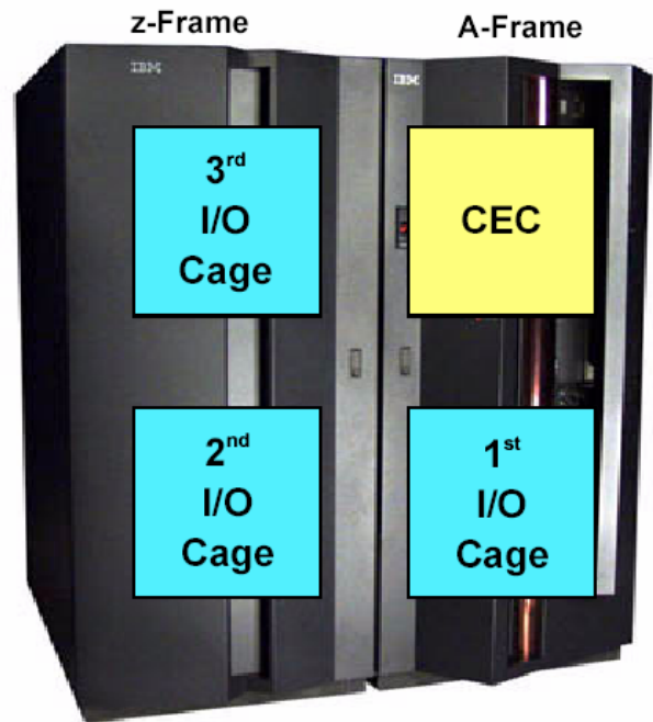
Behind the covers of a 2-frame [i.e. A- and Z-Frame] z990 and a diagram of how the main A-Frame holds the CEC and the 1 st I/O cage while the z-Frame is used to house I/O cages two and three.
