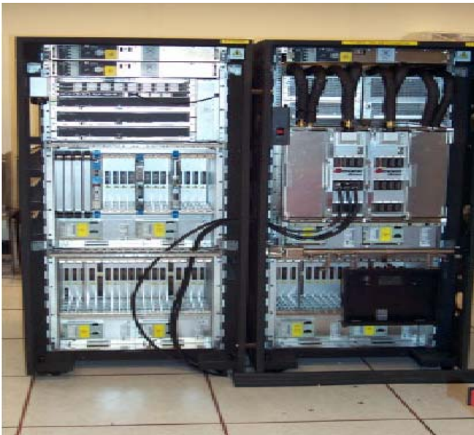
Behind the covers of a 2-frame [i.e. A- and Z-Frame] z990 and a diagram of how the main A-Frame holds the CEC and the 1 st I/O cage while the z-Frame is used to house I/O cages two and three.
