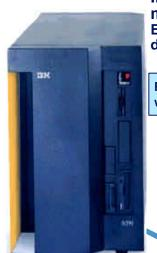
IBM S/390 Multiprise 3000 7060-H50 mainframe with 2GB memory, 24 ESCON channels & 8 parallel channels delivering 120MIPS
